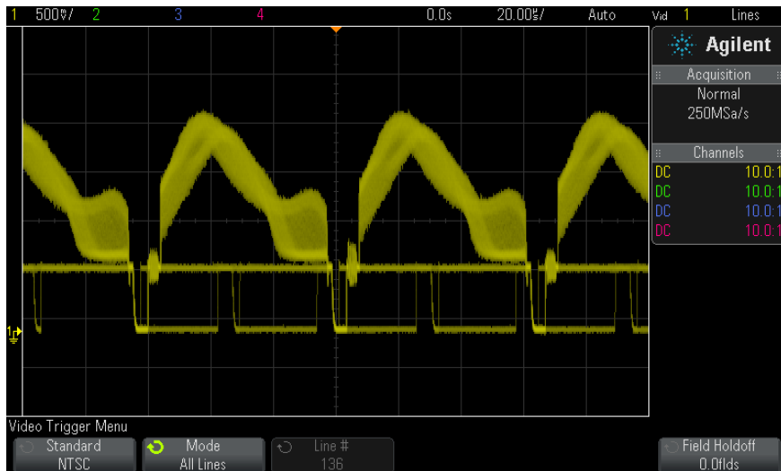
Figure 16 Triggering on All Lines
