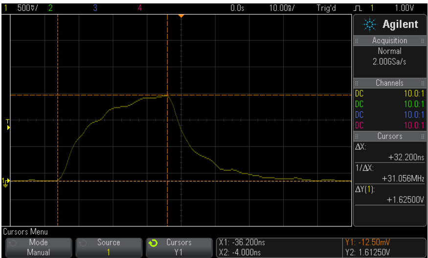
Figure 28 Cursors used to measure pulse widths other than middle threshold points
