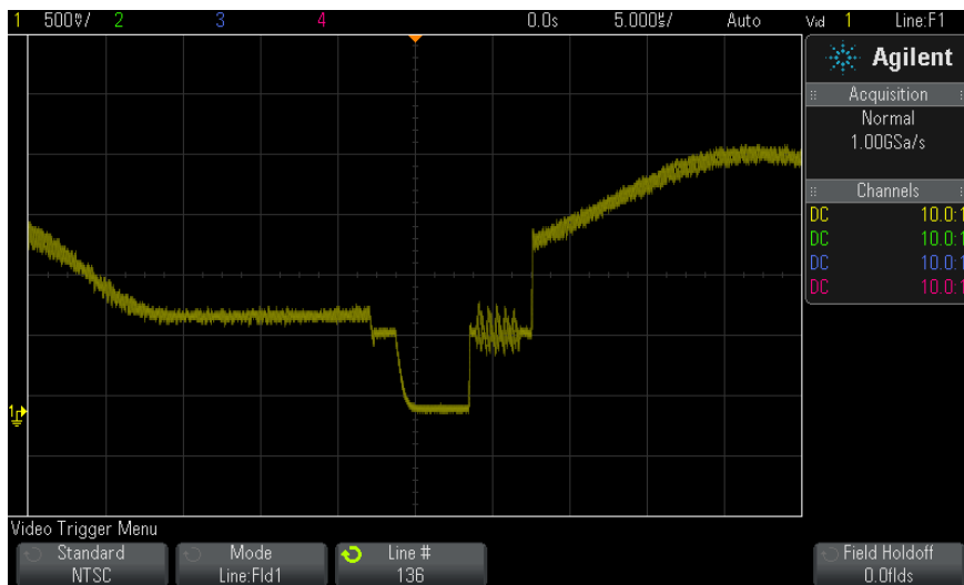
Figure 15 Example: Triggering on Line 136
